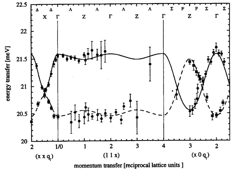
Fig. 2: Measured dispersion of the  $\Gamma_6^{(1)} - \Gamma_6^{(2)}$  - Nd crystal field excitation in  $\text{Nd}_2\text{CuO}_4$  at 4 K (circles:  $q_1=0$ , squares:  $q_1=2$ ). The lines correspond to the RPA model calculation (—: acoustic branch, ---: optical branch).
