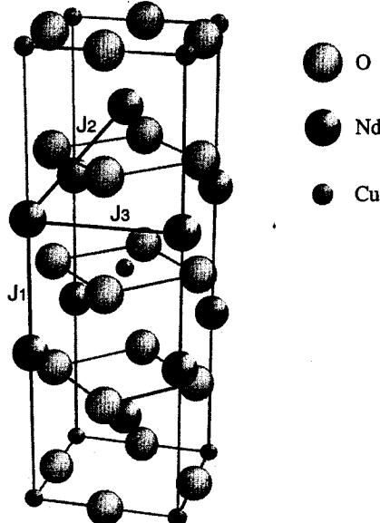
Fig.4: Crystal structure of  $\text{Nd}_2\text{CuO}_4$  with the various Nd-Nd exchange constants indicated.
