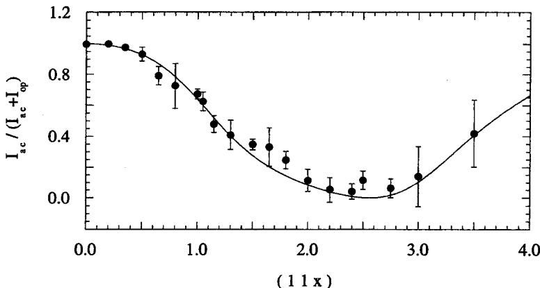
Fig. 3: Measured intensity of the acoustic branch at (11x) positions, normalized to the total magnetic scattering. The line corresponds to the RPA model calculation.
