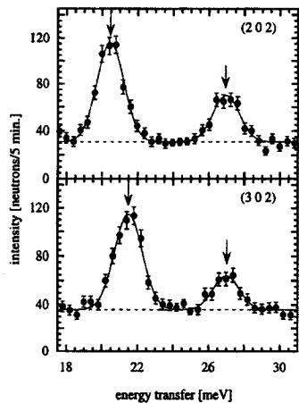
Fig. 1: Energy spectra of neutrons scattered from  $\text{Nd}_2\text{CuO}_4$  at 4 K at two different  $\bar{Q}$ -positions.
