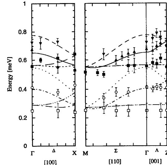
Fig. 6: Measured dispersion of the Nd spin waves in  $\text{Nd}_2\text{CuO}_4$ . The lines correspond to the model calculation with the exchange constants given in the text.
