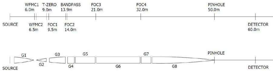
Figure 5: First layout of the baseline model for the neutron transport system of ODIN. G1 is the bi-spectral feeder. G2 and G3 are the elliptical expansion part of the ballistic guide. G4, G5, G6 and G7 are the straight sections. G8 is the guide that focuses the neutrons at the pinhole. 10 meters after the pinhole, the detector will be placed. All the gaps between guides are to house the required choppers.
