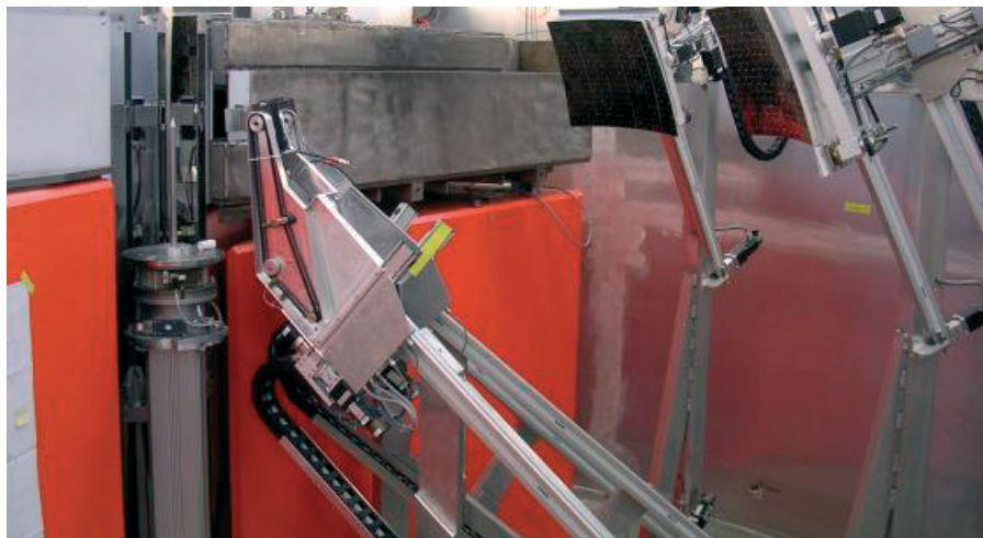
Figure 12: Analyzer and detector banks of the backscattering spectrometer MARS at SINQ
