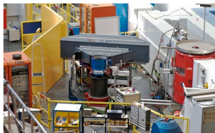
Figure 18: High-intensity multidetector powder diffractometer DMC@SINQ for cold neutrons at SINQ.
