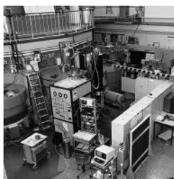
Figure 15: 7 mK refrigerator used 1988 on the two-axis neutron diffractometer P2AX@SAPHIR.
