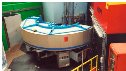
Figure 20: High-resolution powder diffractometer HRPT@SINQ for thermal neutrons with multidetector and electronics.
