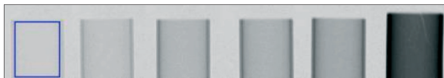
Figure 3: Calibrated fuel cladding samples with well-known hydrogen content imaged at BOA.
