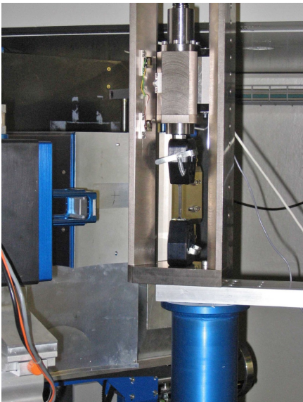
Figure 2: The tensile machine on the POLDI sample table. In the background the radial collimator is visible, on the right site the adjustable slits for the incident beam.
