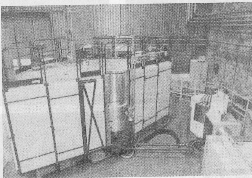
Overview of major hardware components of FOCUS. From left to right: Ar-filled flight chamber containing 400 ^3\text{He} -filled detectors. Then the sample chamber, Fermi-chopper, monochromator shielding, focusing guide and lead filled biological shielding.
