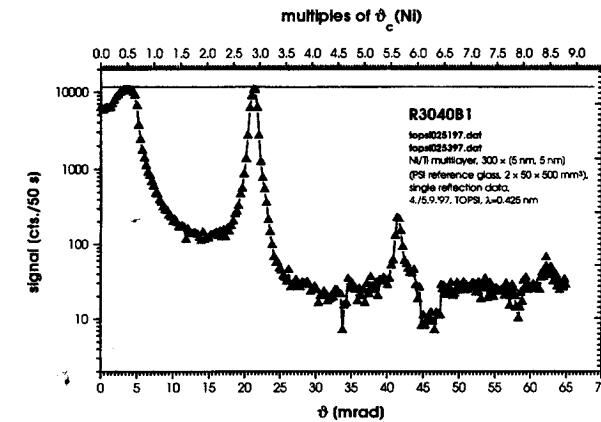
Fig.1. Reflectometry data of a  $\text{Ni}/\text{Ti}$  bilayer
