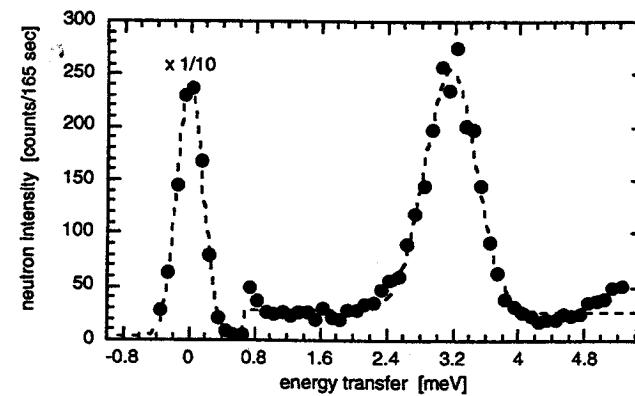
Energy spectrum of neutrons scattered from TmNi<sub>2</sub><sup>11</sup>B<sub>2</sub>C.
