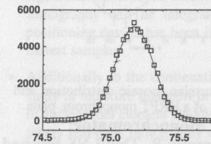
**Fig. 2:** Rocking curve of a single  $\text{Ge}_{311}$ -slab measured at TOPSI/ SINQ using a perfect Ge-monochromator.
