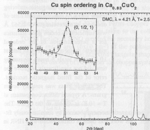
examples of clear evidence for Cu spin ordering obtained by powder neutron diffraction. These measurements have been performed in collaboration with IBM, Rüschlikon.
