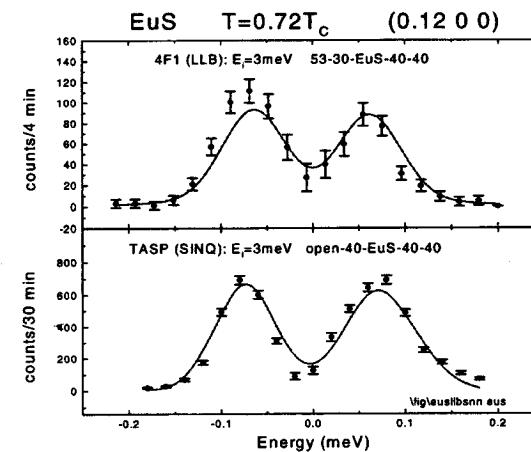
**Fig. 2:** Spin waves in EuS at small  $q$ .
