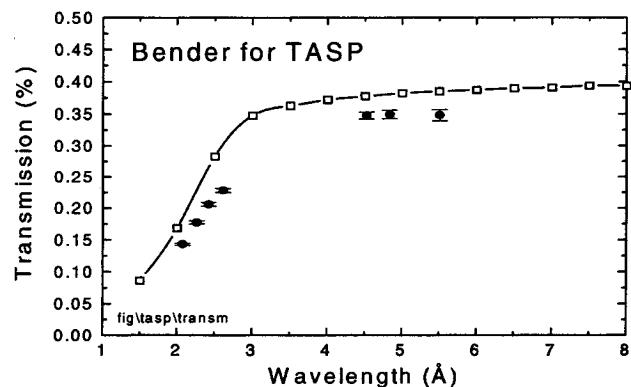
**Fig. 1:** Calculated transmission of the short polarising benders. The filled circles indicate the measured transmission for different neutron wavelengths.
