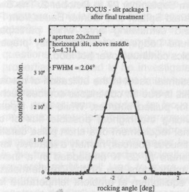
Fig. 1: Rocking curve of the Fermi-Chopper collimation package
