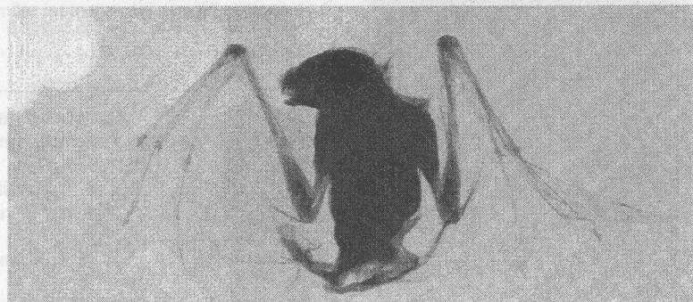
Fig. 1: The image of a bat illustrates the good ability of neutrons to investigate organic samples and biologic objects.
