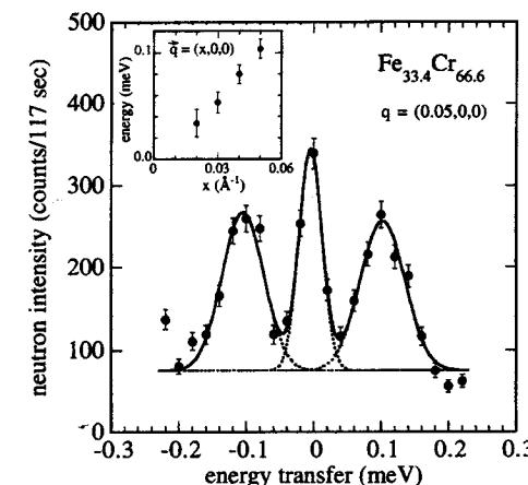
Fig. 1: Energy spectrum of neutrons scattered from  $\text{Fe}_{33.4}\text{Cr}_{66.6}$ . The inset shows the dispersion curve of magnons at small momentum transfer.
