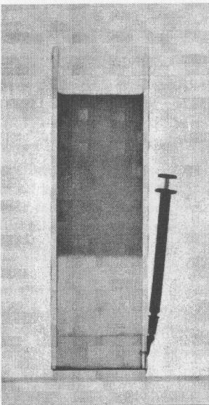
**Fig. 2:** The behaviour of light (above) and heavy (below) water as layers inside the case was investigated. Such measurements can be performed easily with NR only. The stability of the border was studied over several hours. Beside the qualitative impression also the numerical information is available for the description of the processes.
