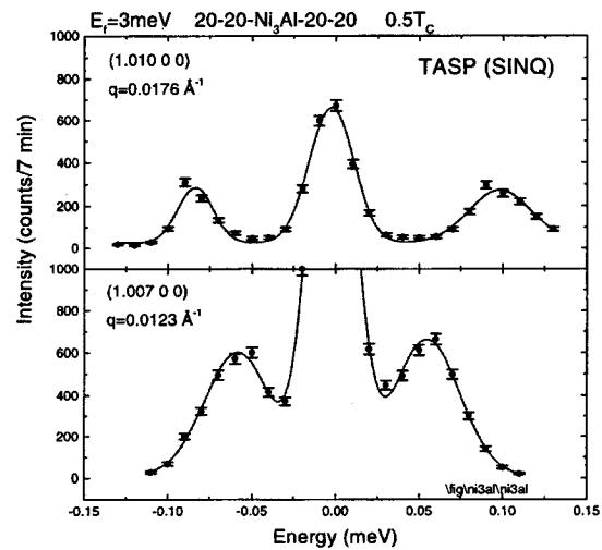
Fig. 3: Spin wave excitations in single crystal  $\text{Ni}_3\text{Al}$  at  $T=20\text{K}$ .
