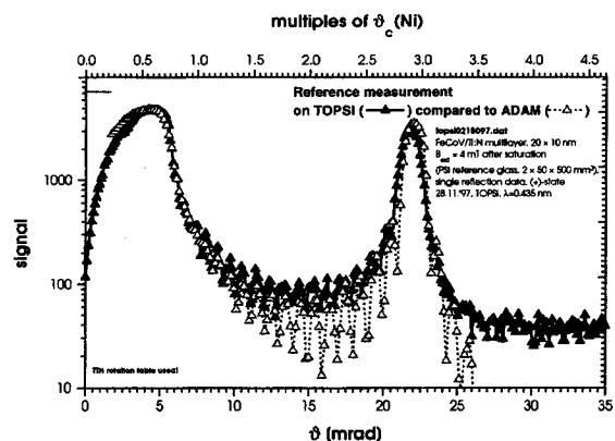
Fig. 2. Polarised reflectometry data of a FeCoV/Ti bilayer
