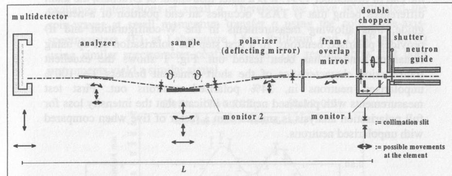
Sketch of the overall instrumental layout of the PSI reflectometer. Components for the generation of magnetic fields, positioning aids, and single detectors are omitted.
