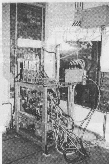
**Figure:** The inner helium circuit of the rabbit systems (for sample transport and cooling) is perfectly separated from the outer atmosphere by helium tight slides, developed by PSI. The entry of the transport channel into the target block can be seen in the centre of the picture. The remote controlled system is operated inside a concrete shielding.
