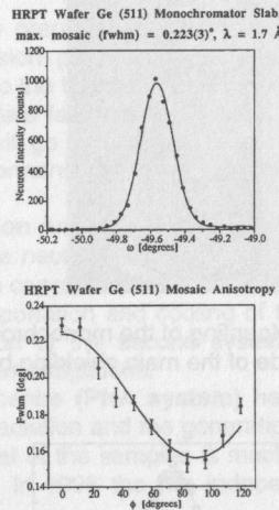
Fig. 2: Gaussian mosaic distribution and anisotropy of a HRPT monochrom. plate
