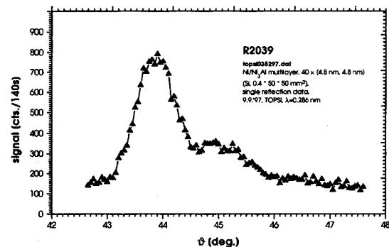
Fig. 3. High angle diffraction data of a Ni/Ni<sub>3</sub>Al bilayer
